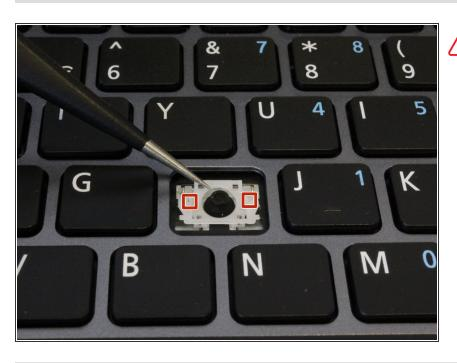
⚠ If the white plastic horizontal spring becomes misaligned, re-align and pop the two hinges back into place with the tweezers or your fingers.
