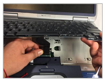
Lift the keyboard and unplug it out of the socket.
