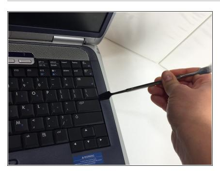
Once all the screws are taken out of the top portion of the keyboard, wedge open the keyboard on all sides of the keyboard.
