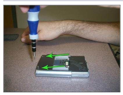
The arrows indicate two small screws. Using a Phillips head screwdriver, remove them.
