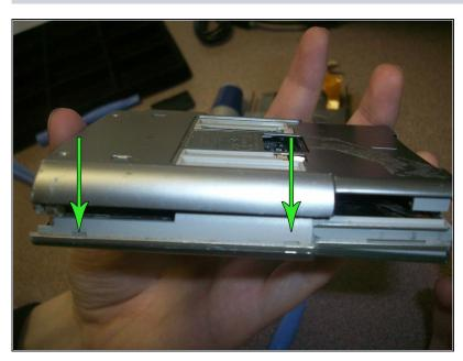
Hint: There will be pressure points along the side (as seen in the picture). Exerting pressure in these points will allow the sides to separate more easily.
