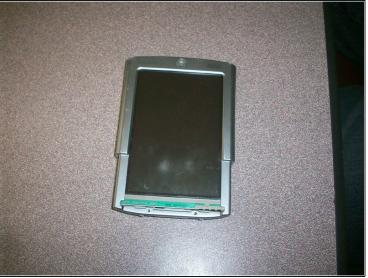
Lay the face plate on device. It must be snapped into place.
