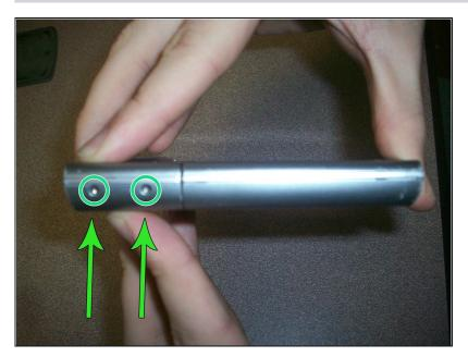
There will be a set of 2 screws located on each side of your device. Remove these by using a Phillips head screwdriver.
