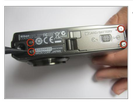
Remove the four 3.2 mm screws on the bottom of the camera.
