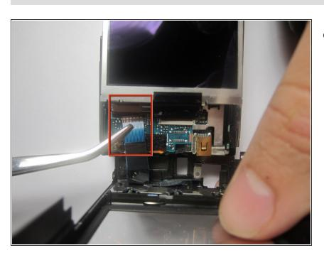
Use the tweezers to disconnect the ribbon from the circuit board.
