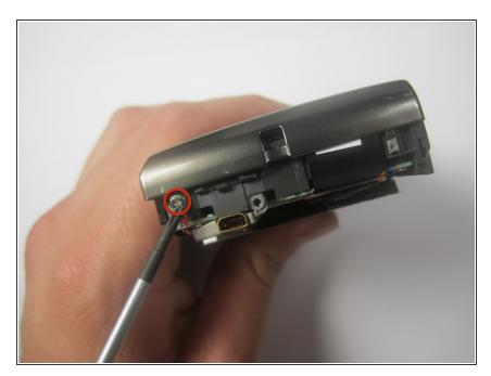
Remove the one 2.6 mm screw from the left side of the camera (with the lens facing forward)
