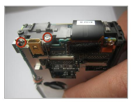
Remove the two 3.4 mm screws from the side of the camera.
