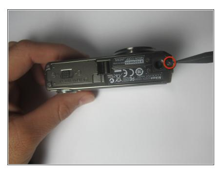
With the lens facing forward, remove the one 4.2 mm screw on the bottom right hand corner of the camera.
