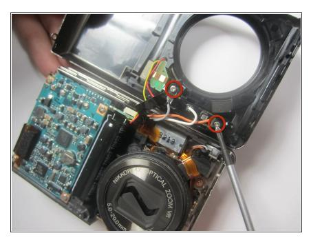
Remove the two 3.2 mm screws that hold the flash to the front cover.
