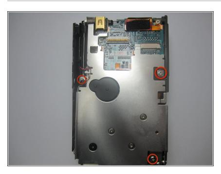
Remove the three 3.4 mm screws from the back side of the camera.
