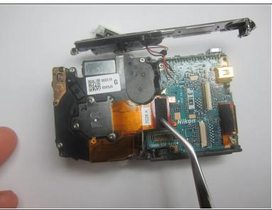
Gently remove the two ribbons connecting the lens to the mother board.
