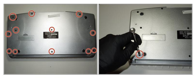
• Remove the 8 mm M3 Phillips head self tapping machine screws.
