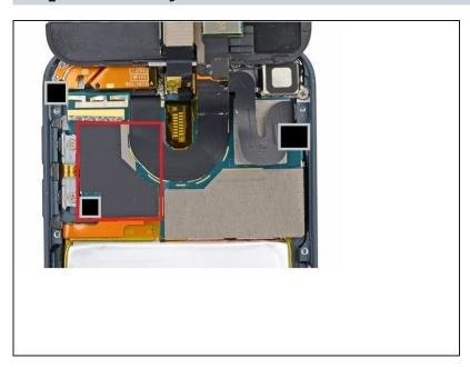
Remove the covering over the battery by applying heat
