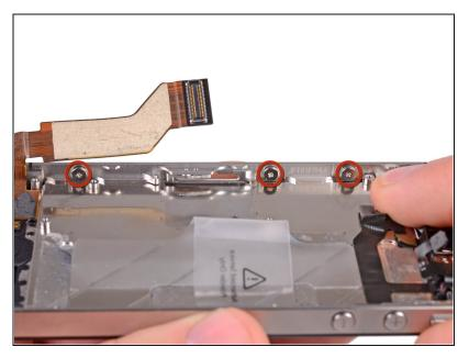
Loosen the three large-headed Phillips screws along the other side of the iPhone about one half turn.
