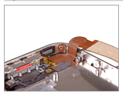
Remove the 1.5 mm Phillips screw near the dock connector cable.
