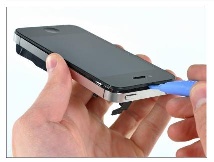
Use the edge of a plastic opening tool to gently pry up the display assembly around its perimeter.
