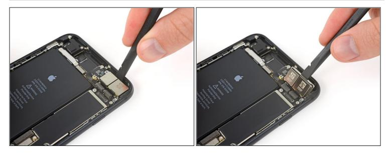
• Use the flat end of a spudger to pry up the rear-facing camera assembly from the top edge of the iPhone.
