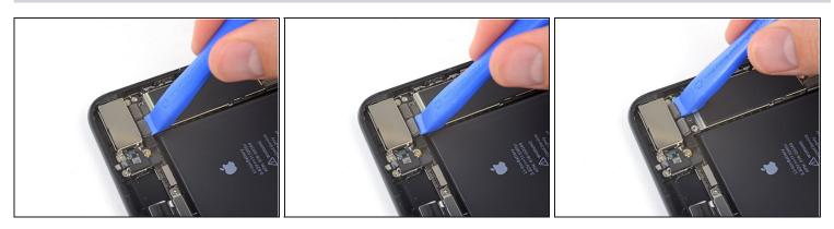
• Use an iFixit opening tool or a fingernail to disconnect the two camera cable connectors by prying them straight up from their sockets.
