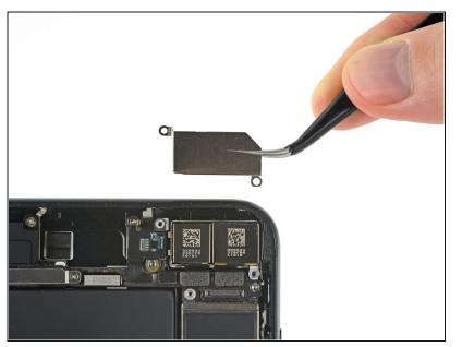
Remove the bracket covering the rear-facing camera assembly.
