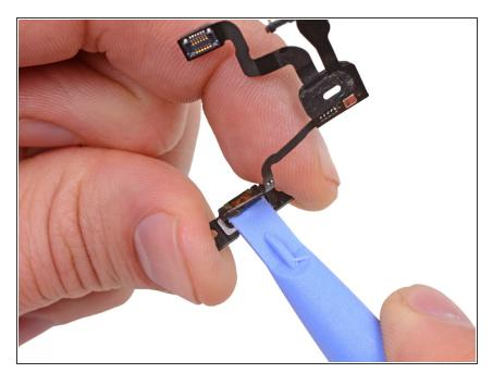
Use the edge of a plastic opening tool to separate the power button contact from its plastic bracket.
