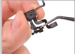
Lift and remove the power and sensor cable assembly from the iPhone.
