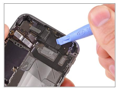
Use the edge of a plastic opening tool to disconnect the Wi-Fi antenna from the logic board.
