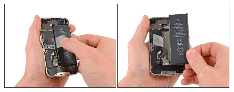
• Use the exposed clear plastic pull tab to peel the battery off the adhesive securing it to the iPhone.
