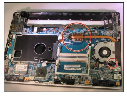
Locate and remove the 6.7 mm screws that hold the fan assembly.
