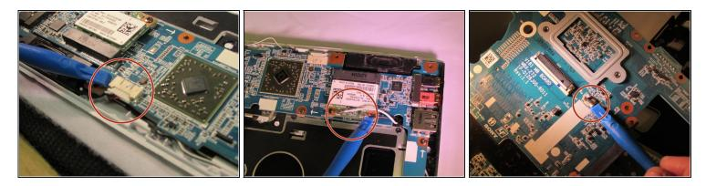
• Locate the wires and connectors and remove them from the motherboard.
