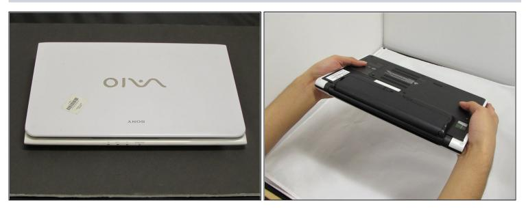
A Remove the charging adaptor. Some charge may still be in the battery or computer. DO NOT touch connectors or copper yellow connector.
