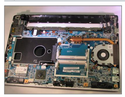
• Gently lift the fan assembly up and out.
