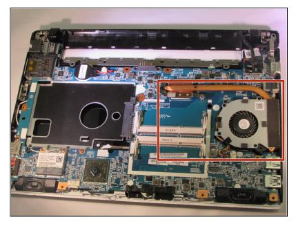
• Locate the fan and heat-sink.
