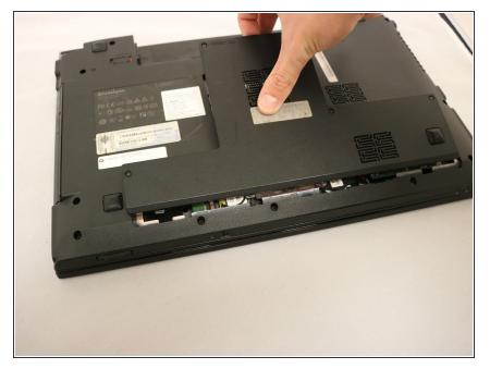
Pull the panel outward from the rest of the laptop. The inside of the laptop will be exposed. From here you can access the CD-ROM drive, hard drive, and Keyboard.
