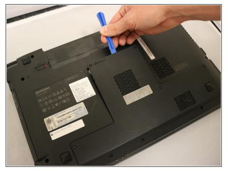
• Using a plastic opening tool, pry the back panel from the laptop.
