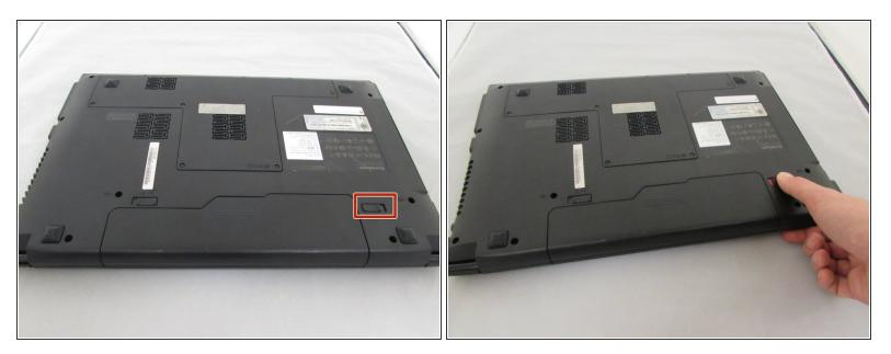
• Push the right-hand switch outward into the "unlocked" position.
