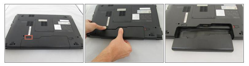
While holding the battery, use your other hand to push the left clip to the left and pull the battery out.
