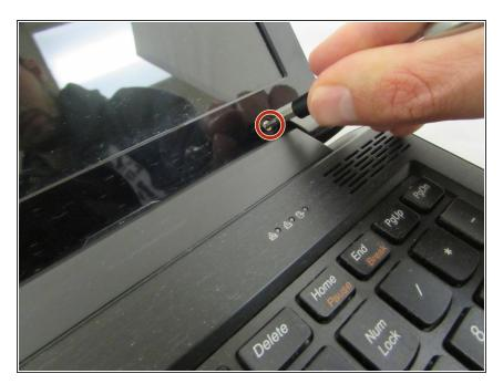
Using the Phillips #0 Screwdriver, remove the two 4.3 mm screws holding the display to the front bezel.
