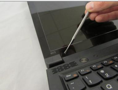
Remove both screw covers from the bottom of screen bezel using a plastic spudger. The screws underneath will now be exposed
