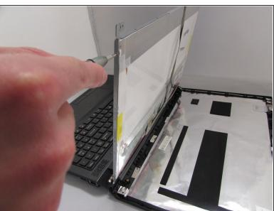
Using the Phillips #0 Screwdriver, remove the four 2.9 mm screws from each side of the bracket that holds the display panel in place.
