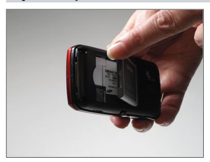
• Carefully remove the battery from the phone.
