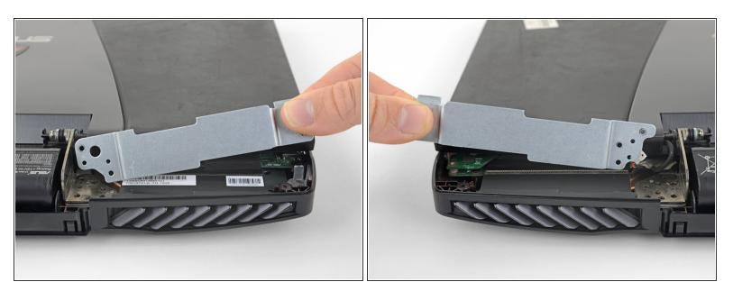
Lift up and remove the two metal display brackets.
