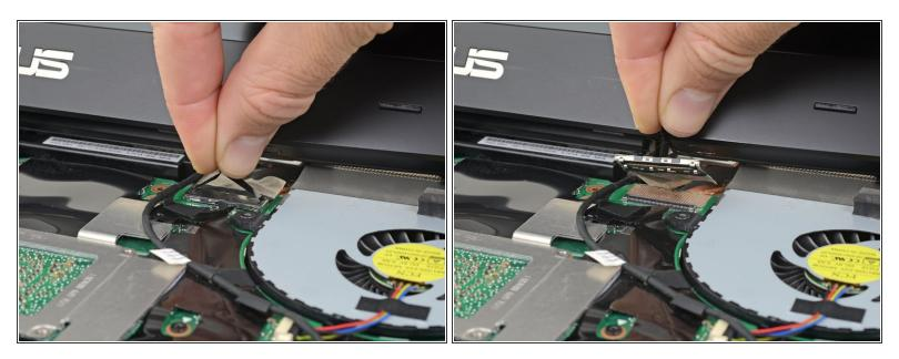
Grab the black tape attached to the display cable and pull straight up to disconnect the display cable.
