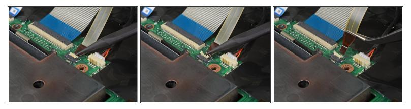
Use the tip of a spudger to flip up the small locking flap of the keyboard backlight cable <u>ZIF</u> <u>connector</u>.
