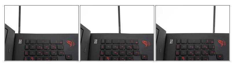
Slide the spudger along each edge of the upper case assembly, prying and releasing clips as you go.
