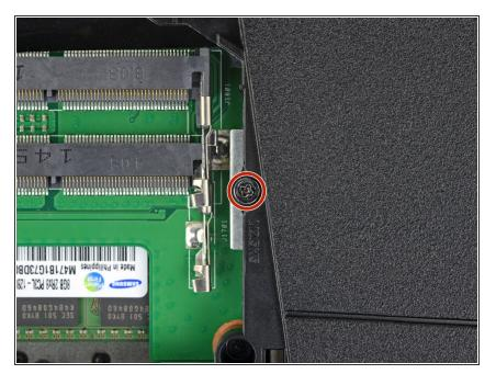
• Remove the 5.2 mm Phillips #00 screw securing the optical drive.
