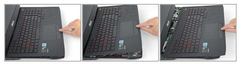
• When all the clips securing the upper case assembly have been released, lift the assembly slightly and slide it down, away from the display, about an inch.
