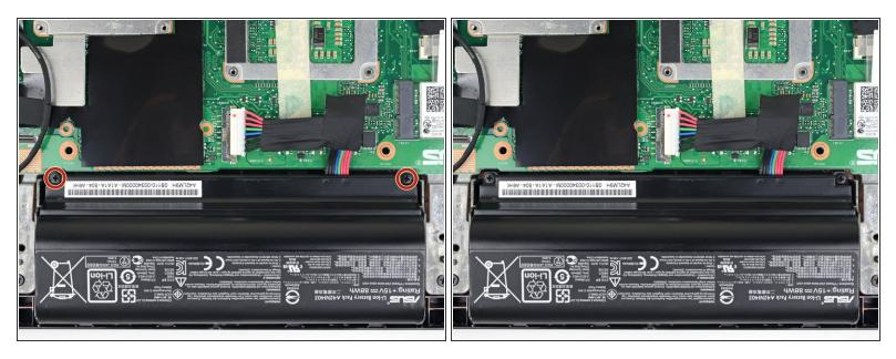
Remove the two 5.7 mm Phillips #00 screws securing the battery.
