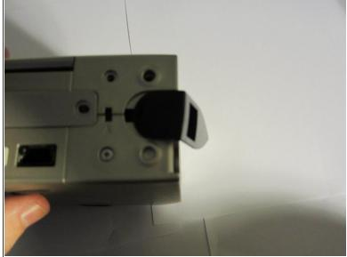
Push down and slide the tabs on both sides of the back of the printer away from the device to remove the tabs.
