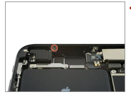
• Remove the 1.3 mm Phillips screw securing the antenna component to the top edge of the rear case.
