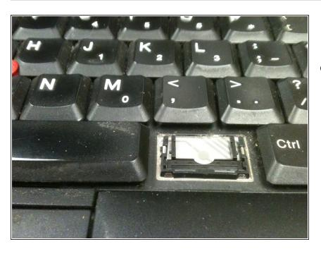
The new key will have an empty slot where they key used to be. It contains a small rubber spring. After the rubber spring is inserted take the new key and line it up according to the color springs on the backside of the key along with the keyboard.
