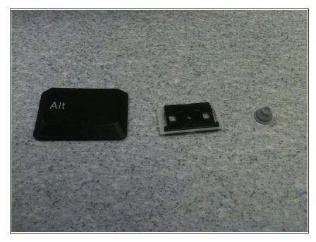
Step 3: Set the old key aside and have the new key ready to be inserted onto the computer. The key has three parts, which you can see here.
