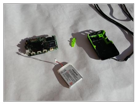
Unplug the logic board from the battery. Replace the logic board with your new logic board and reassemble your device.
