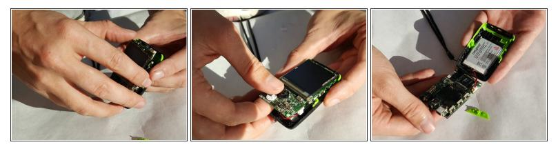
• Pull up on the motherboard and display. It is glued to the base so it will require a little force. Be careful though, as the board is fragile.
