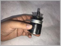
Unscrew the torque adjuster from the transmission by removing the screws highlighted in the lefthand picture.
