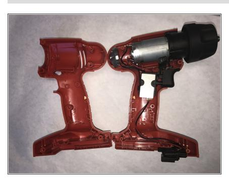
Separate the outer drill case to expose the components and switch.
