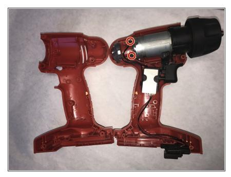
Reconnect black and red wires onto the motor and place the motor, transmission and torque adjuster back onto their initial location.
