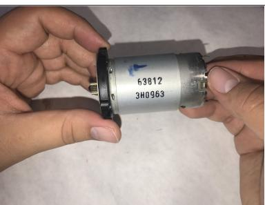
Remove the motor from the transmission assembly, as pictured.
