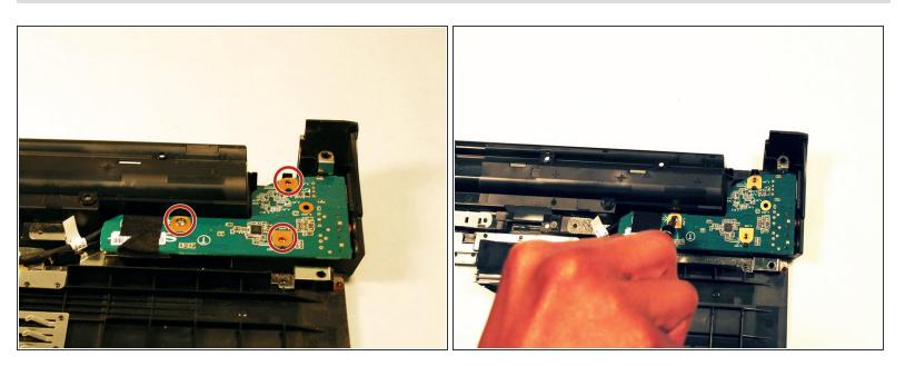
Remove the screws holding the headphone jack board down.
