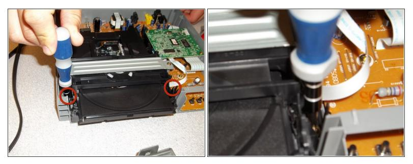
• Use a Phillips #2 screwdriver to remove the two screws at the base of the disk drive.
