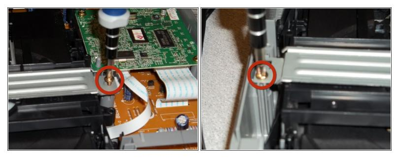
Use the screwdriver to remove two screws on either side of the silver security bar.
