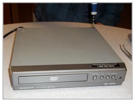
• Use a Phillips #2 screwdriver to remove the two screws on the top of the device toward the back.
