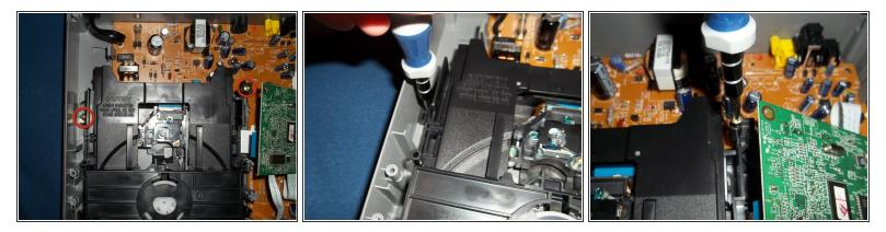
• Remove the two screws at the back of the disk drive.
