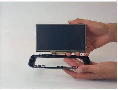
Begin by removing the flaps pressing LCD screen against device. Then, detach screen from the adhesives by gently pushing on the screen and disconnect remaining yellow flap from screen.
