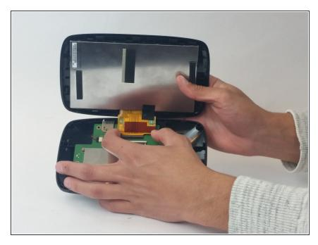
Disconnect the screen from the motherboard by removing the flap connecting both with your hands.
