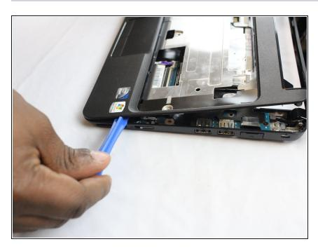
Lift the keyboard bezel from the back end and slide the iFixit opening tool around the perimeter of the bezel until it is fully released.
