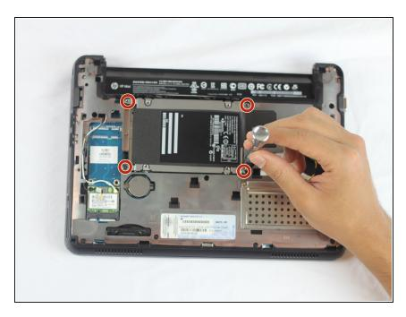
Remove the four screws holding down the hard drive using a Phillips #1 screwdriver.
