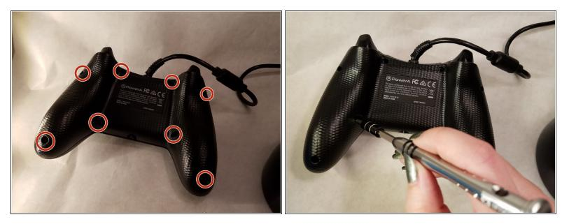
Disassemble the case by removing the 8 screws, indicated in red on the picture, that hold the back
