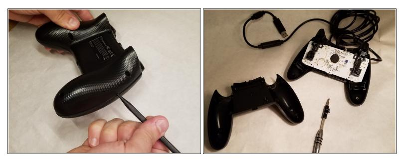
• The case should come apart easily. If not, use a spudger to pry the back from the front of the case.
