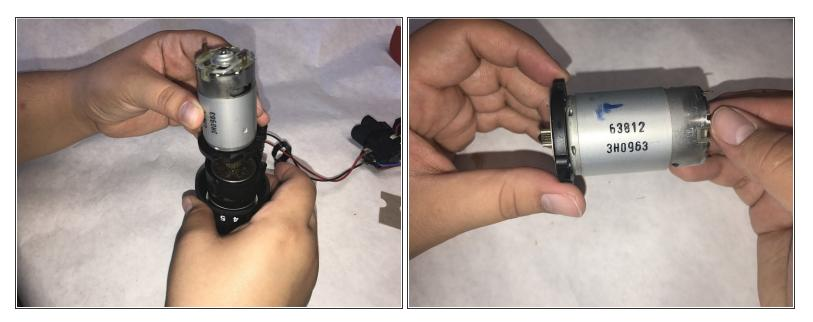
• Remove the motor from the transmission assembly, as pictured.
