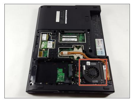
The cooling fan is located near the edge of the device, on the side with the vent, and is contained within a plastic shroud.
