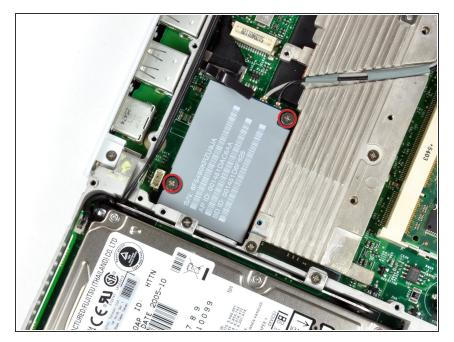
Remove the two 3 mm Phillips screws securing the AirPort card to the logic board.
