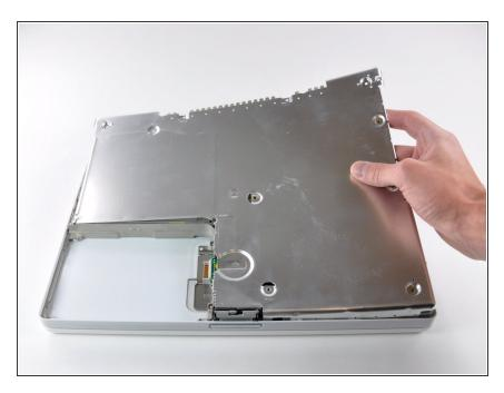
• Lift the bottom shield off.
