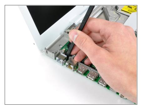
Wedge a spudger between the RJ-11 board and the metal framework and slide the board to the left, off of the logic board.
