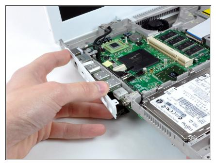
• Lift up the left side of the computer and slide the I/O bezel away.
