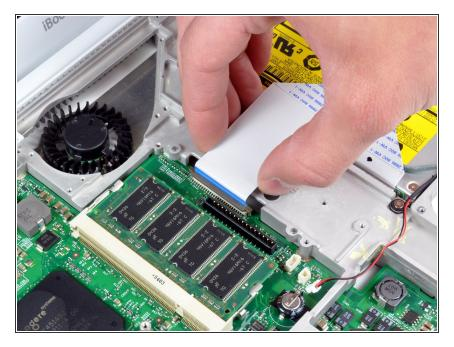
Release the optical drive ribbon clamp as described above. Slide the optical drive ribbon out of its connector.
