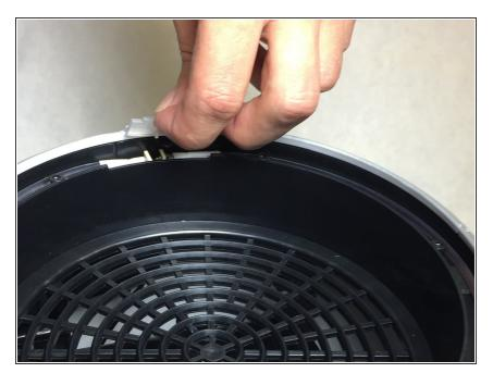
After lifting 45 degrees, pull the translucent tab away from thee housing. Repeat this step for the second LED cover.
