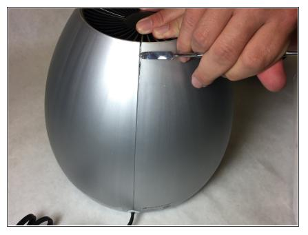
• Locate the tab about 1 inch below the top vent. Insert a flat tool laterally past the tab and press in toward the center of the device. As the tab is being held down, pull the two halves of the egg apart to keep the shell open.
