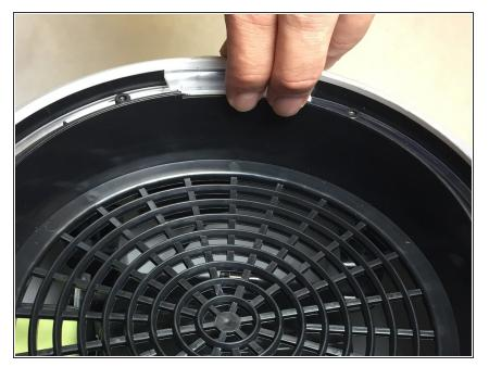
Using two fingers lift the translucent LED cover from the inside. Repeat this step for the second tab.
