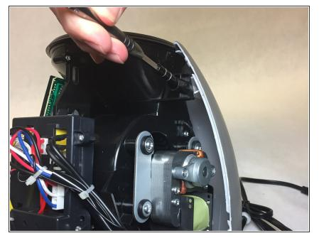
• Locate the screw housing opposite of the control board, and remove the screw.
