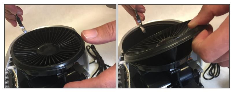
• Use a flathead tool to place it in between the the exhaust vent and the inner side of the outer shell.
