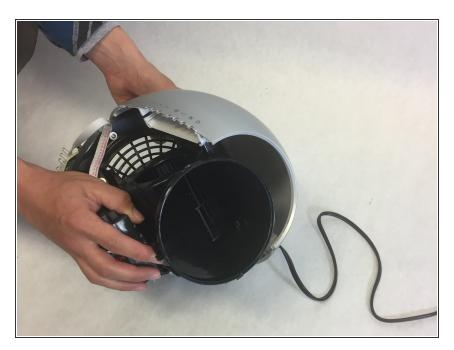
Remove the released half of the shell to finish removing the entire outer shell of the device.
