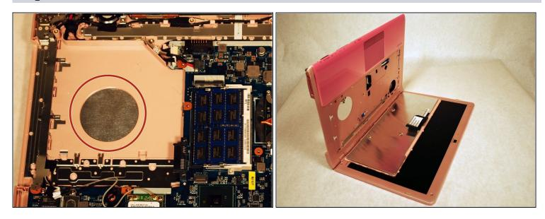
• With the laptop open, gently push on the silver circle shown. This is the back side of the keyboard and will cause the keyboard to pop out.
