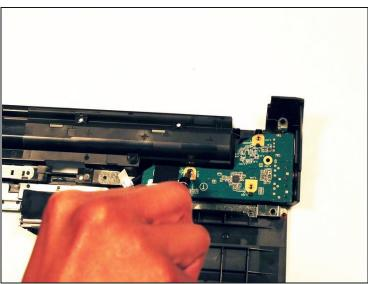
Remove the screws holding the headphone jack board down.
