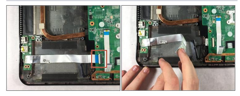
• Carefully disconnect the cable connecting the ports to the motherboard from the right side.
