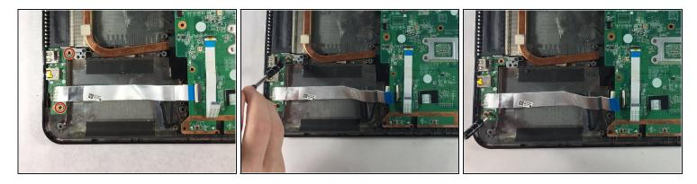
Remove the two 6.0 mm screws from the ports.
