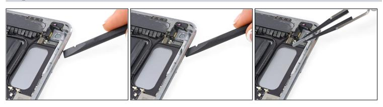
• Using a spudger or your finger, press in on the top and bottom button cover to remove them.
