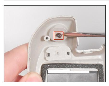
Use a metal spudger to push the button out of its socket so that you can place a new one in its place.
