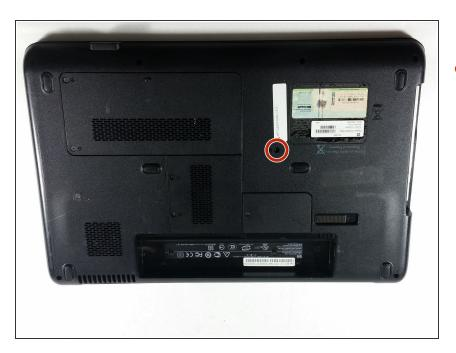
Unscrew the 5mm screw holding the CD player in place.
