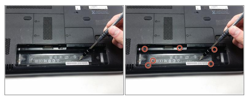
Unscrew the following 5mm screws with a #0 Phillips screwdriver.
