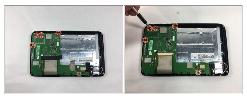
Unscrew four screws in the top left corner by using Phillips #0 size screwdriver.
