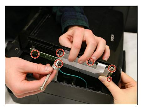
Remove the six 3mm Phillips #2 screws connecting the control panel to the circuit board.
