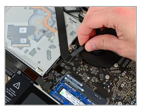
Use the flat end of a spudger to lift the AirPort/Bluetooth connector out of its socket on the logic board.
