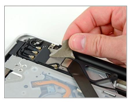
Peel back the piece of EMI tape covering the AirPort/Bluetooth cable on the AirPort/Bluetooth housing.
