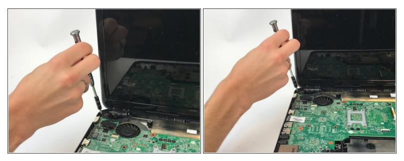
• Next, unscrew the two 7.25mm screws in the upper left corner of the laptop as shown.
