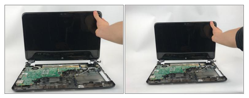
Once all of the screws have been removed, gently lift the laptop's screen from the base of the computer.
