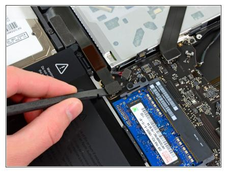
Disconnect the hard drive/IR sensor cable from its socket on the logic board by lifting up from beneath its connector.
