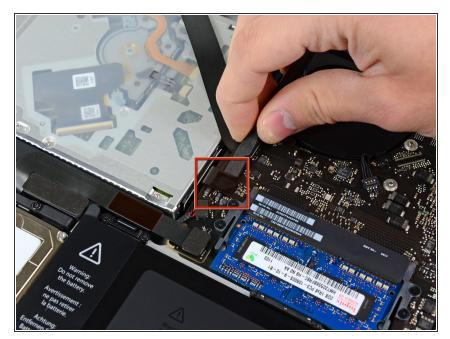
• Use the flat end of a spudger to pry the optical drive connector up from its socket on the logic board.
