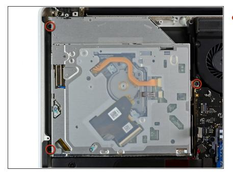
Remove the three 3.5 mm T6 Torx screws securing the optical drive to the upper case.
