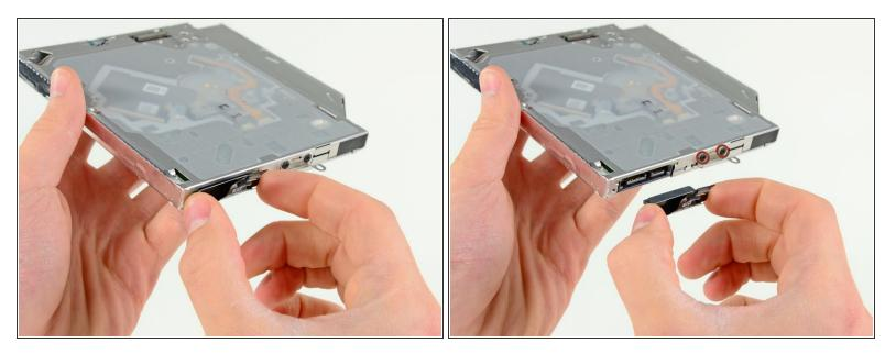
• Pull the optical drive cable out of the optical drive.
