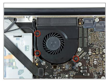
Remove three T6 Torx screws securing the right fan to the logic board and upper case.
