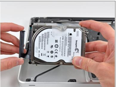
Pull the hard drive connector out of its socket on the hard drive.
