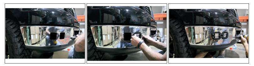
Insert in your new LED Pod Lights and screw it in tightly to your truck.
