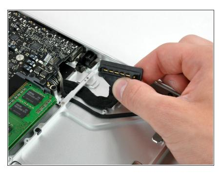
Peel the battery connector cable off the adhesive securing it to the upper case.
