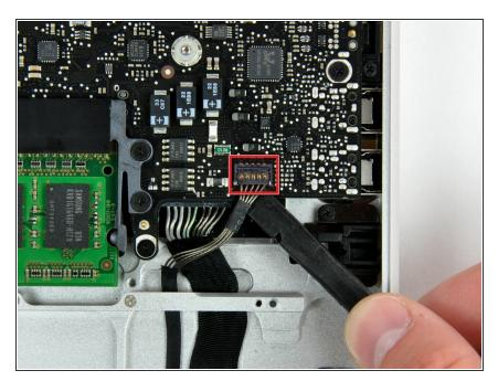
Using a spudger, pry the battery level indicator cable connector straight up off the logic board.
