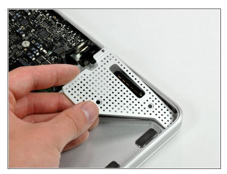
Lift the battery connector cover out of the upper case.
