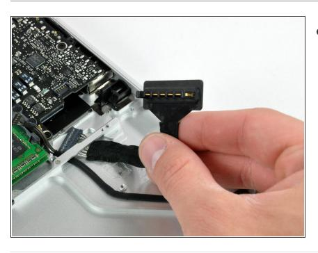
De-route the battery connector cable through the gap in the upper case and remove it from the computer.
