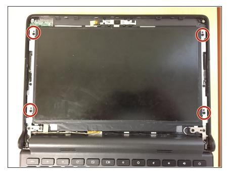
• Remove the 4 LCD screws in each corner of the screen. Make sure to just unscrew the 4 corner screws as the other screws are not needed.
