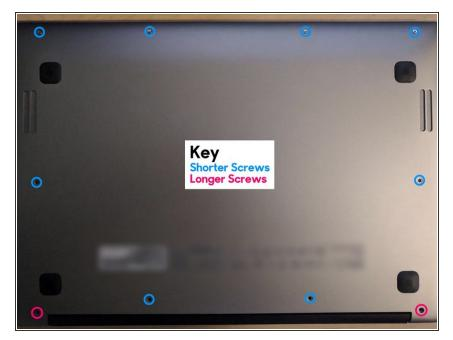
After unscrewing these philipsheads the back panel pops right off with no adhesive, no ribbons attached too!
