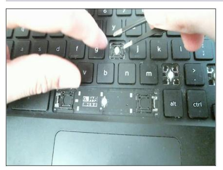
With tweezers, carefully start picking near the four corners where the 4 metal clips are securing the plastic bracket.
