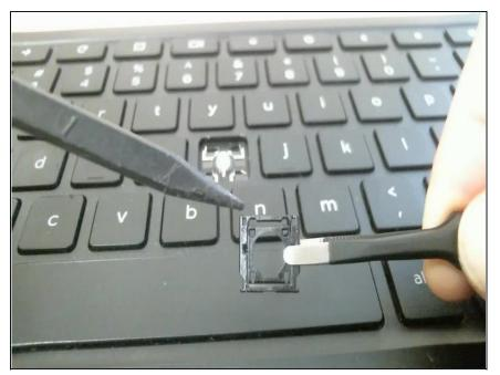
• Line up the 2 outer corners and the bottom inner corners of the plastic bracket with the 4 metal clips connected to the palmrest.
