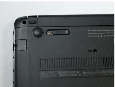
Set the lock switch to the orange unlocked position.
